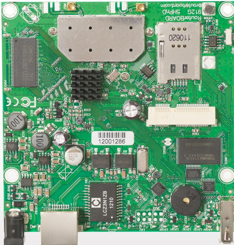
The RB912 is a small wireless router with an integrated high power wireless card and an additional miniPCIe slot for 802.11 wireless, or 3G card. Both 2GHz and 5GHz models are available. The Gigabit port helps to utilize the full potential of 802.11n wireless speeds.
